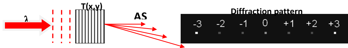
Figure 1. Diffraction on phase grating described by function T(x,y) and imaging of diffraction pattern using AS.
