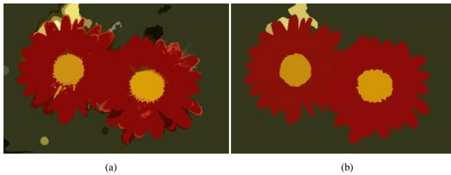
Fig. 5. Segmented and ground-truth images: (a) segmented image from Figure 1, K = 55 ; (b) ground-truth segmentation, K_{GT} = 9 .
