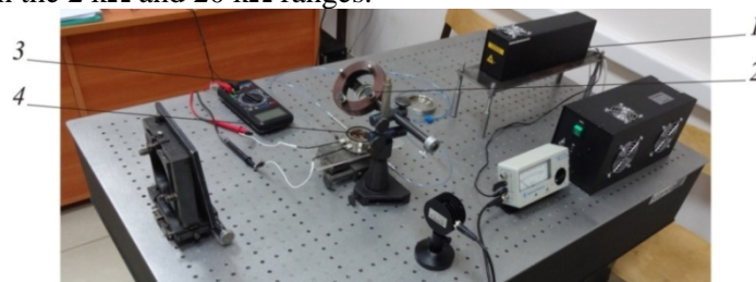
Figure 6. The experimental setup for determination the dependence of CNT-sample resistance on the laser beam power: 1 – laser, 2 – mirror, 3 – multimeter, 4 – CNT-sample on a substrate.
