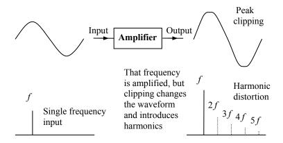
**Harmonic Distortion.** A common type of amplifier distortion is called harmonic distortion. It can arise if any component in the amplifier clips the peaks of the waveform. A common specification for high fidelity amplifiers is the total harmonic distortion. This distortion may be less than 1%. or even less than 0.5% from 20-20,000 Hz for high quality amplifiers.
