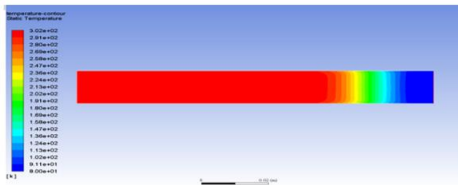
Fig. 1 – Static temperature contour of conventional straight pulse tube model
