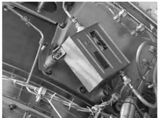
Fig. 7. Ignition unit installation
