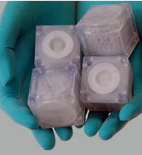
Microsatellite with four control moment gyroscopes
