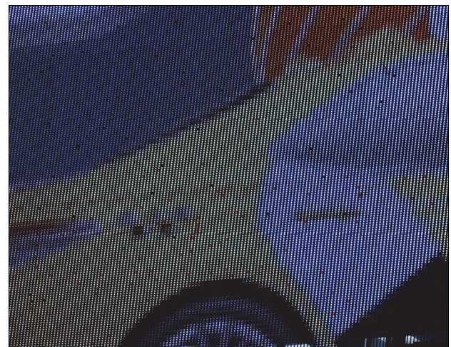
Fig. 1. Defective pixels on large format LED-array display can be easily spotted and significantly reduce the quality of the displayed image
